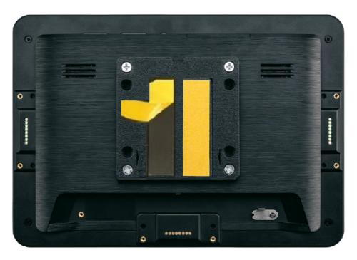
11) Remove the tape from the 2 adhesive strips
